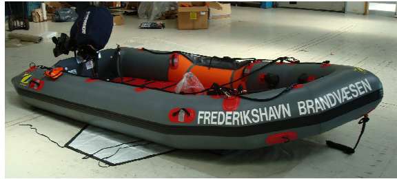
Zodiac MinuteMan with rescuezone. Inflated in 60 seconds by compressed airbottle.
